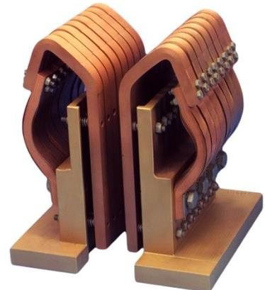
The principle is based on two contact halves which are equipped with spring-mounted movable contact fingers. The mounting distance of the contact halves is thereby less than the thickness of the goods rail so that the contact surfaces can be cleaned by abrasion during the retraction of the goods rail.
