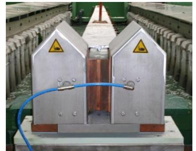
The quality of an electrical connection depends on the material, the cross-section, the dimension and the finishing of the contact areas as well as on the contact pressure. Such facts define the electrical contact resistance and finally the operation and life time of the connection. So when working with a higher contact pressure the electrical resistance will be reduced.
